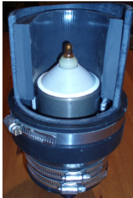
Figure 2.9. Photograph of a Hydrophone Baffled from the Direction of a Spill Gate
