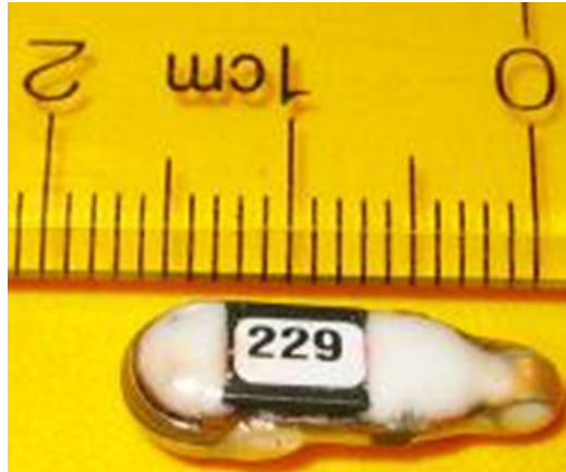
Figure 2.1. Sonic Concepts® JSATS Acoustic Micro-Transmitter
