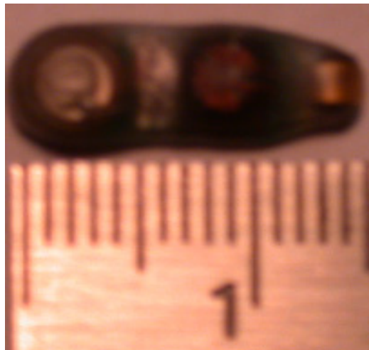
Figure 2.2. The ATS JSATS Acoustic Micro-Transmitter
